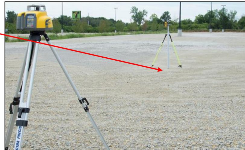
5. Press and release button **E** to open the Grade Match submenu; then press button **E** to start Grade Match (GM Y).
