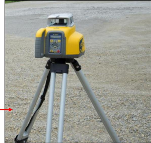
2. Attach the HL760 receiver to a grade rod. Check the laser beam elevation close to the laser.
