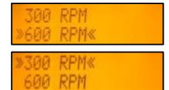
Press and release button **E** to confirm the selected rotation speed.
