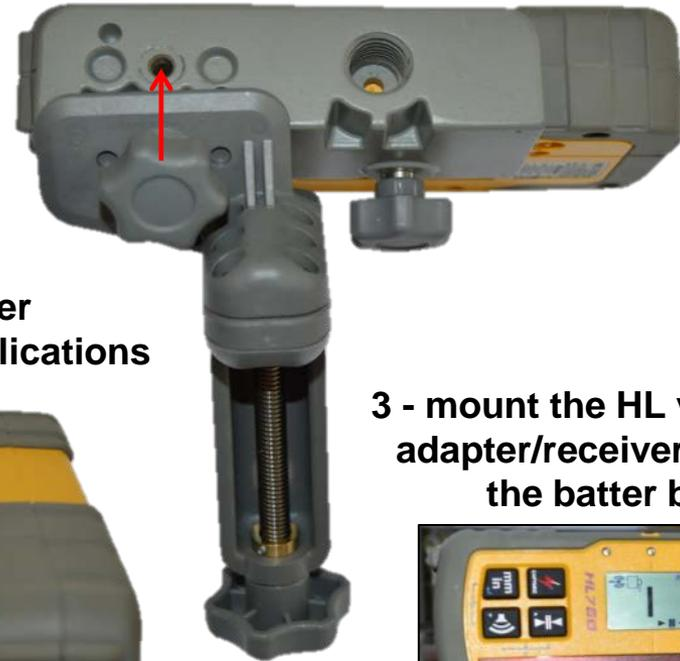
3 - HL vertical adapter/receiver combo ready for vertical applications
