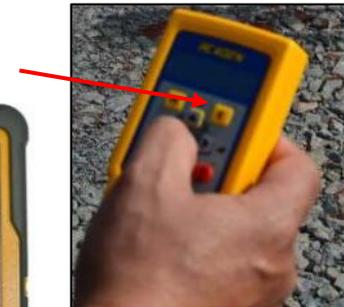
Exiting of PlaneLok can be done by pressing button
