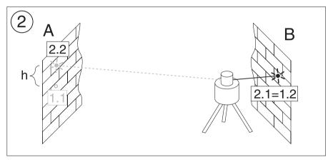
If the unit is within its working accuracy limits ( $\pm$  20") the maximum difference from true level at 20 m (65 ft.) + 20 m (65 ft.) = 40 m (130 ft.) is 4 mm (3/16 inch).
